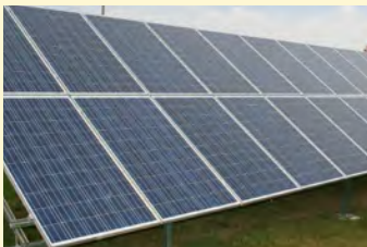
Multicrystalline or polycrystalline solar cells
